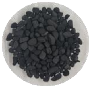
Figure 5.1 - BPL activated carbon granulates, supplied by Chemviron Carbon.
