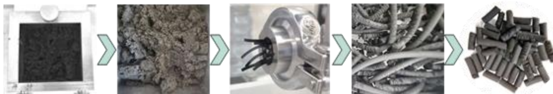
Figure 5.2 - Schematic of the extrusion process of the pelletised Maxsorb AC.
