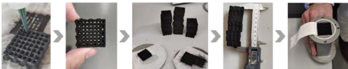
Figure 5.3 - Schematic of the 3D-printing process of a Maxsorb monolith and packing of a column.
