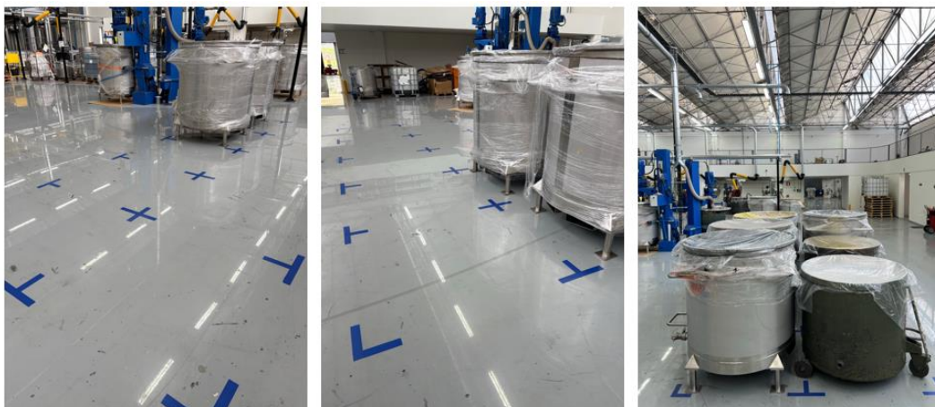
Figure 23 – Mobile tank storage area after 5S implementation
