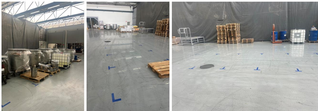
Figure 25 – Supply area after 5S implementation
