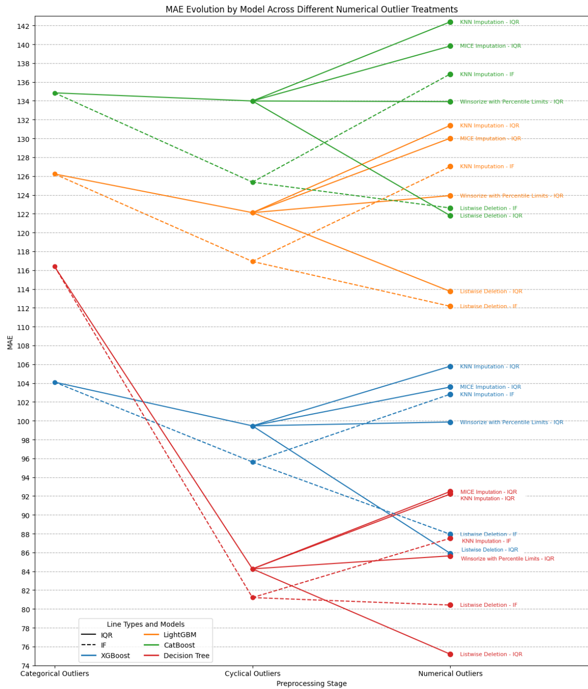
Figure 8.6: Comparative MAE analysis of ML models during categorical outliers removal and different numerical outliers treatment with data from Site 2.
