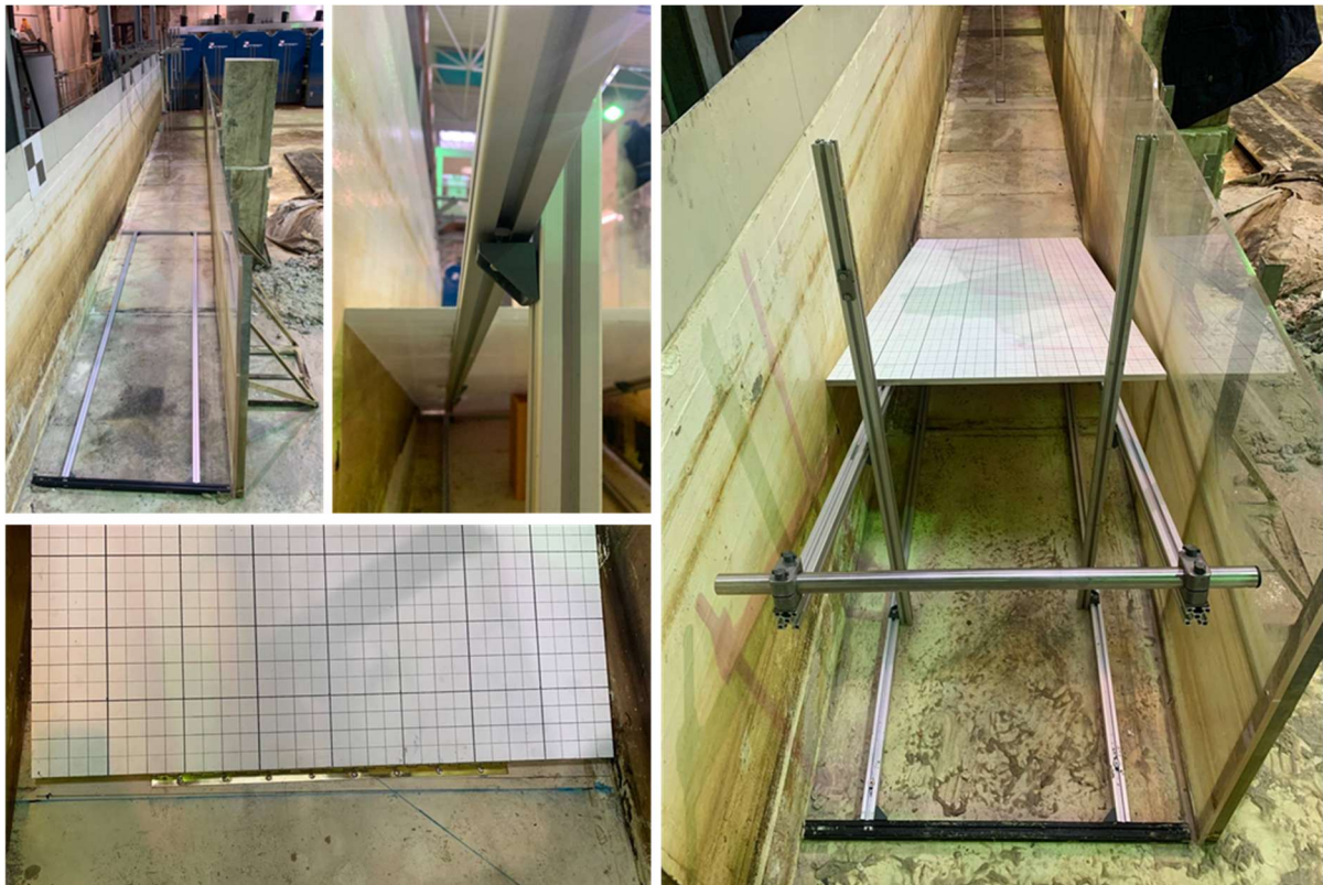
Fig.89 – Side view (top) and top views (bottom) of the model, smooth (bottom left) and rough (bottom middle and right) configurations.
