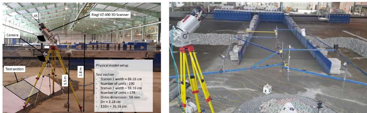
Fig.8 – Laser scanner and fixed camera positioned over the test section (Left side). The model with scanner and calibration box (Right side).
