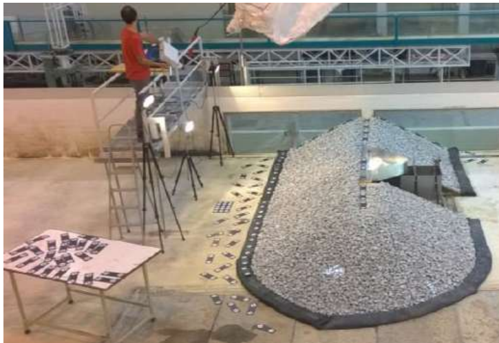
Fig.5 – Damage measurement using the DSP technique (Hofland et al. , 2017).
