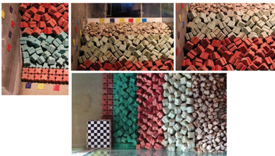
Fig.6 – Setup for two - dimensional scale model tests and targets used in DSP technique (Lemos et al. , 2018).
