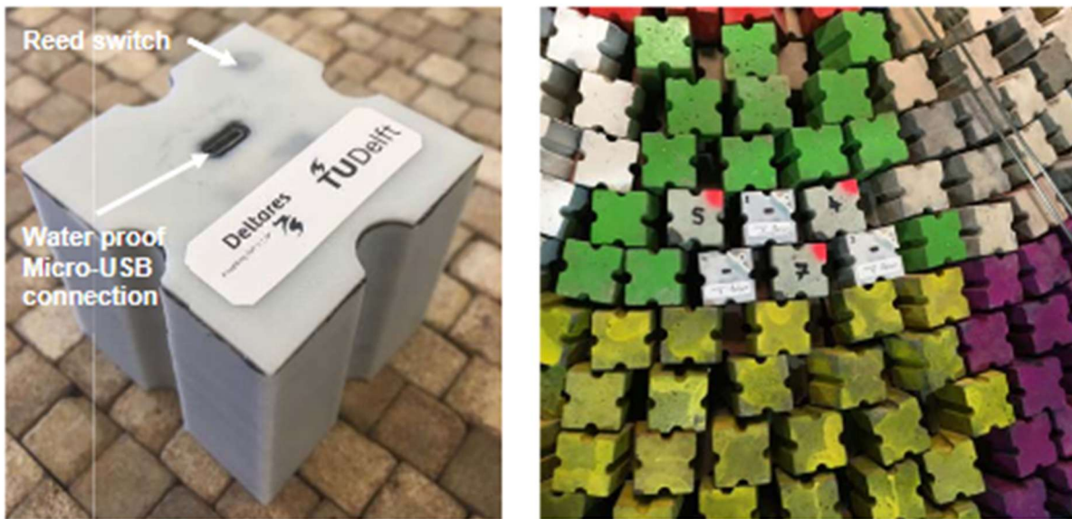
Fig.14 – Model instrumented Antifer unit (left) and instrumented units in the breakwater (right).
