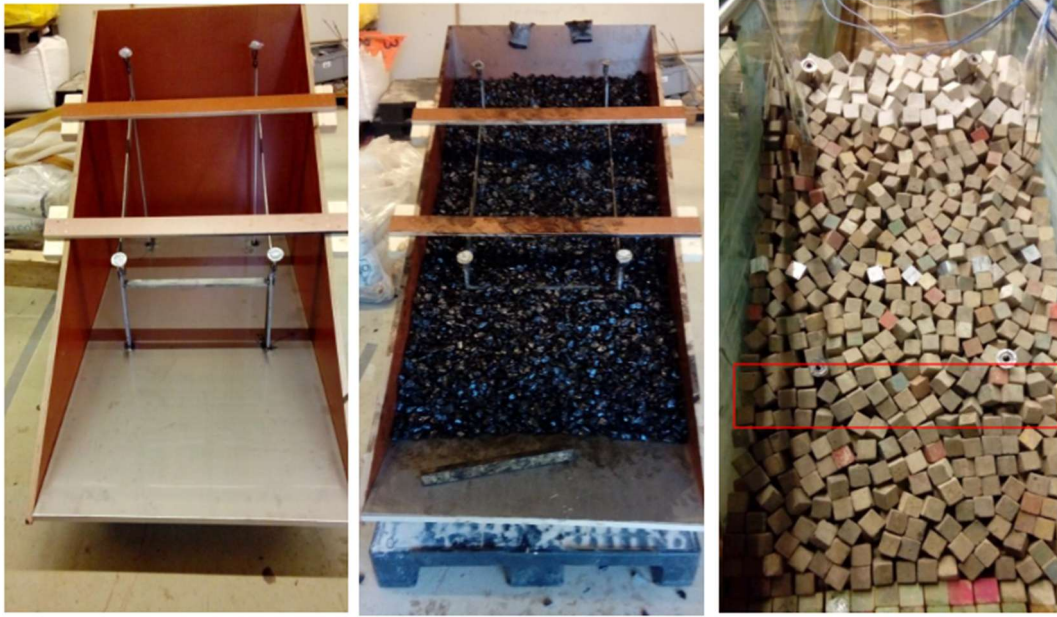
Fig.12 – Model preparation: empty mold for slope preparation (left), prepared slope for testing (middle), and cubes placed randomly in a double layer arrangement (right) (Arefin, 2017).
