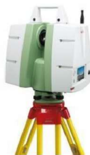
Fig.9 – A Leica C10 Scan Station (Russhakim et al. , 2019).
