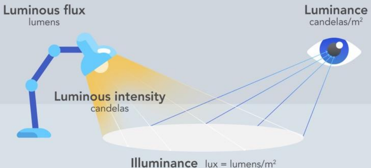
IMG. 4 - How to measure Illuminance (PHILLIPS, s.d.)
