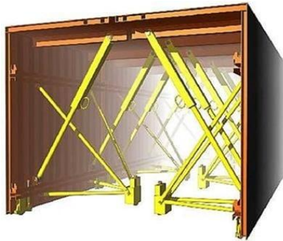
Figure 1: Metallic formwork and supporting elements
