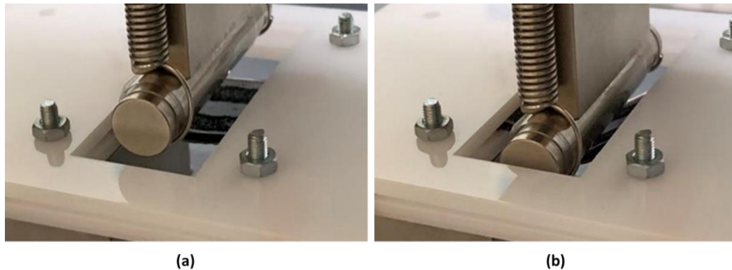
Figure 3.3- Bending tests with an applied force of 6.6 N, a) press and b) release motion.
