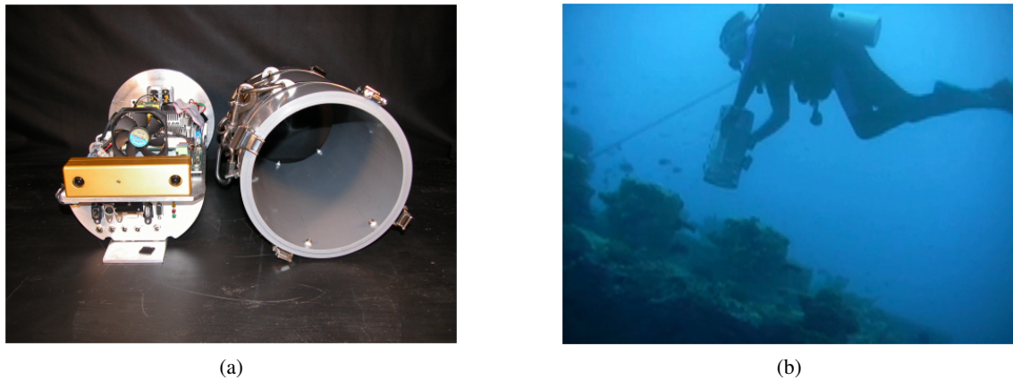
Figure 2.5: The cylinder-shaped AQUASENSOR houses an off-the-shelf stereo camera used by divers for reconstructing and mapping corals and shipwrecks. Extracted from [125].
