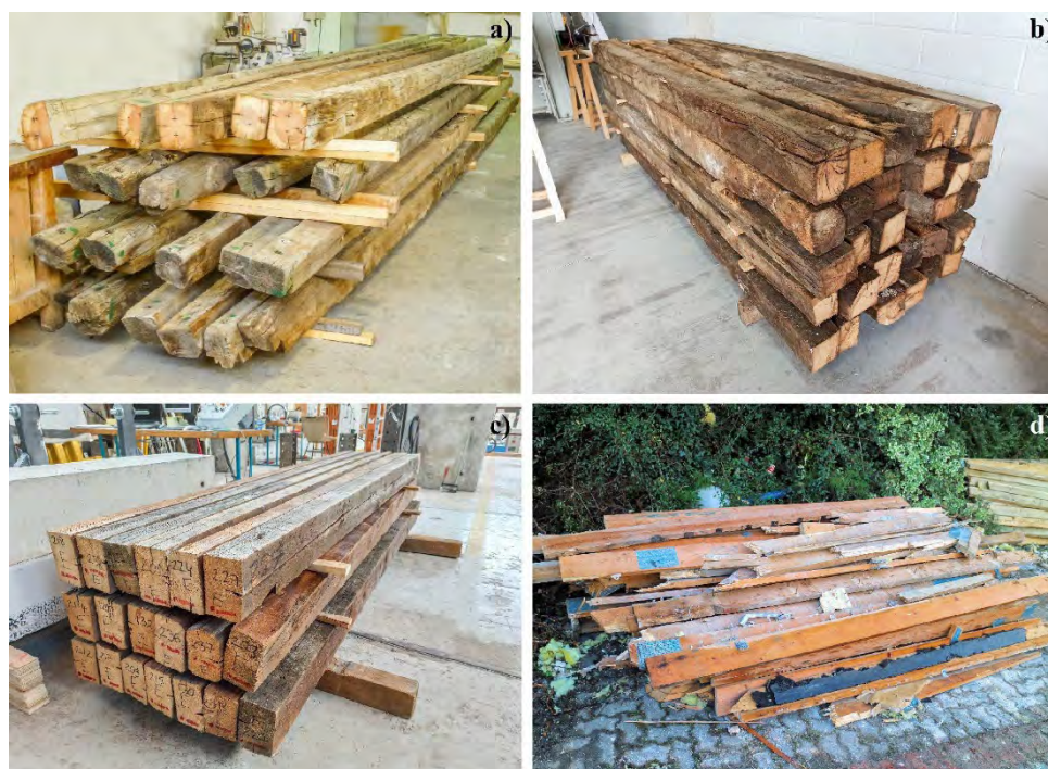
Figure 1. Recovered timber: a) Salzmann pine from 1769, Spain; b) European oak more than 150 years old, Spain; c) Norway spruce from 1949, Slovenia; d) Norway spruce from 1982, Ireland. Source: GICM-UPM.
