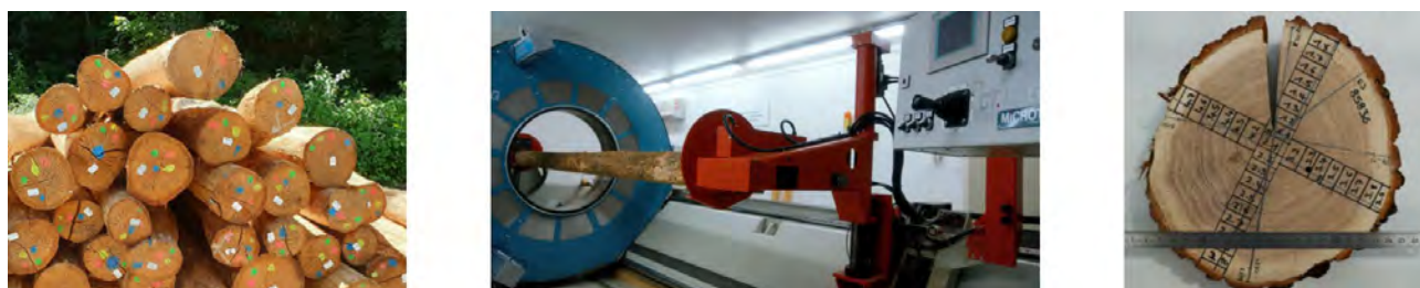
Figure 1. Debarked samples (left), measurement of log density and geometry (middle) and density distribution on a log disc (right).
