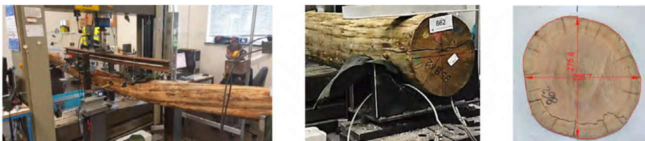
Figure 3. Natural spiral growth and load-induced distortion (left), end-grain with support (middle), digitalized cross-section (right)
