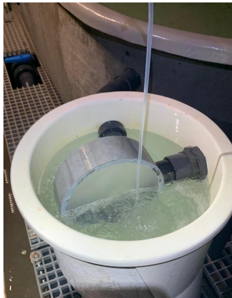
Figure 3 - Egg collector connected to each tank in the Broodstock rooms. Photo taken by Alexandre Veloso.
