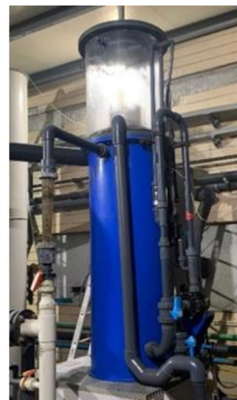
Figure 18 - On the left, protein skimmer schematic from Odd-Ivar Lekang (2013). On the right, protein skimmer used in Safiestela. Photo taken by Alexandre Veloso.
