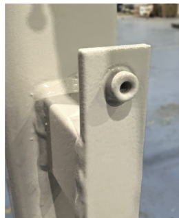
Figure 4.4: Threaded hole with excess paint.
