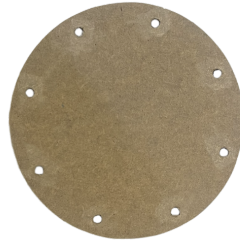
Figure 4.14: Mould for cutting polyethylene from a tank.
