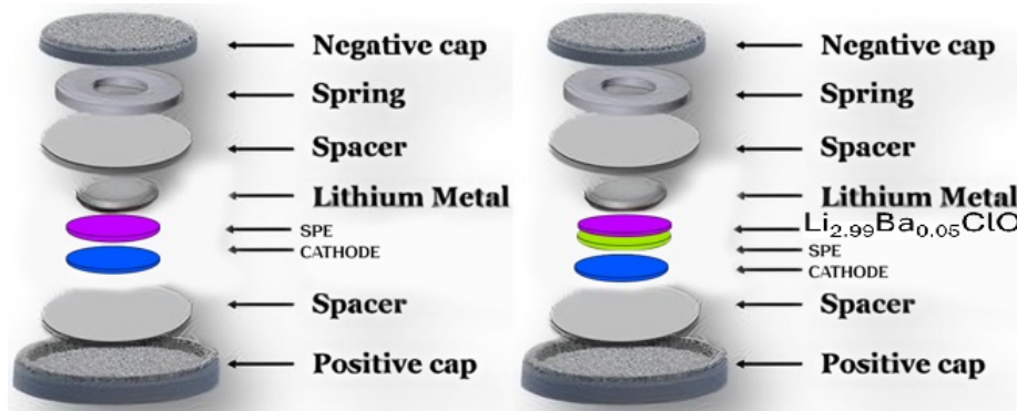
Figure 3.4: On the left: Coin cell using SPE. On the right: Coin cell using SPE and amorphous glass ferroelectric electrolyte ( \text{Li}_{2.99}\text{Ba}_{0.005}\text{ClO} ).
