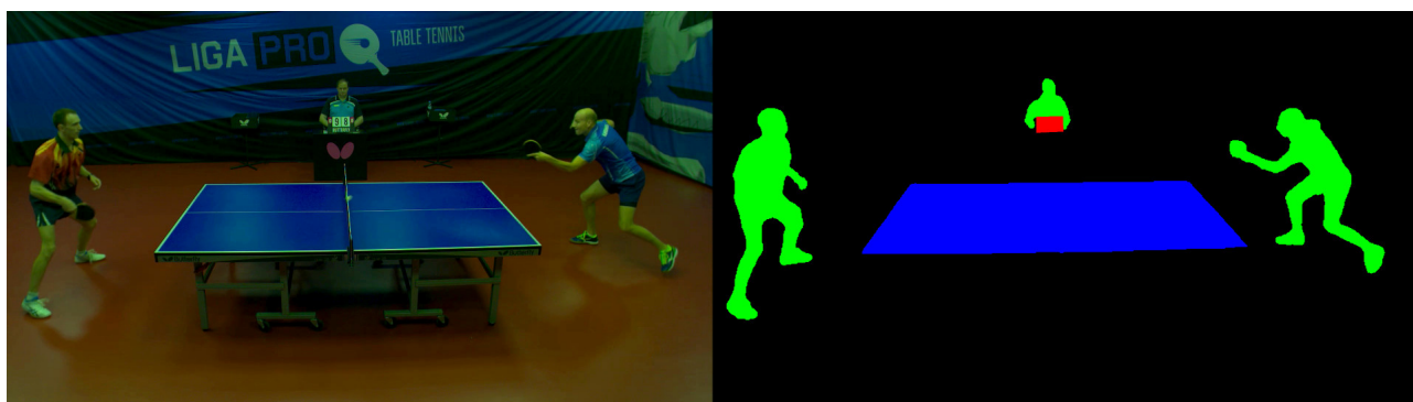
Figure 3.6: Example of a frame with corresponding segmentation masks [38]
