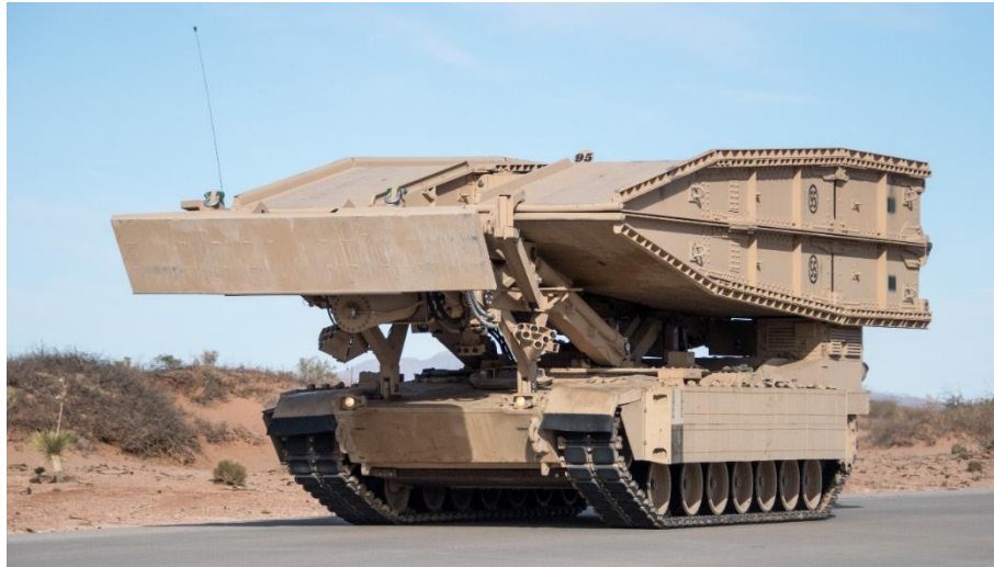
Fig. 2.4 - Ponte JAB – Joint Assault Bridge (U.S. Army 2019)
