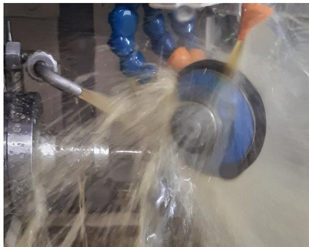
Figure 4- Flooded lubrication while the workpiece is being manufactured.
