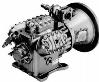
Figure 12: Open type reciprocating compressor [13]
