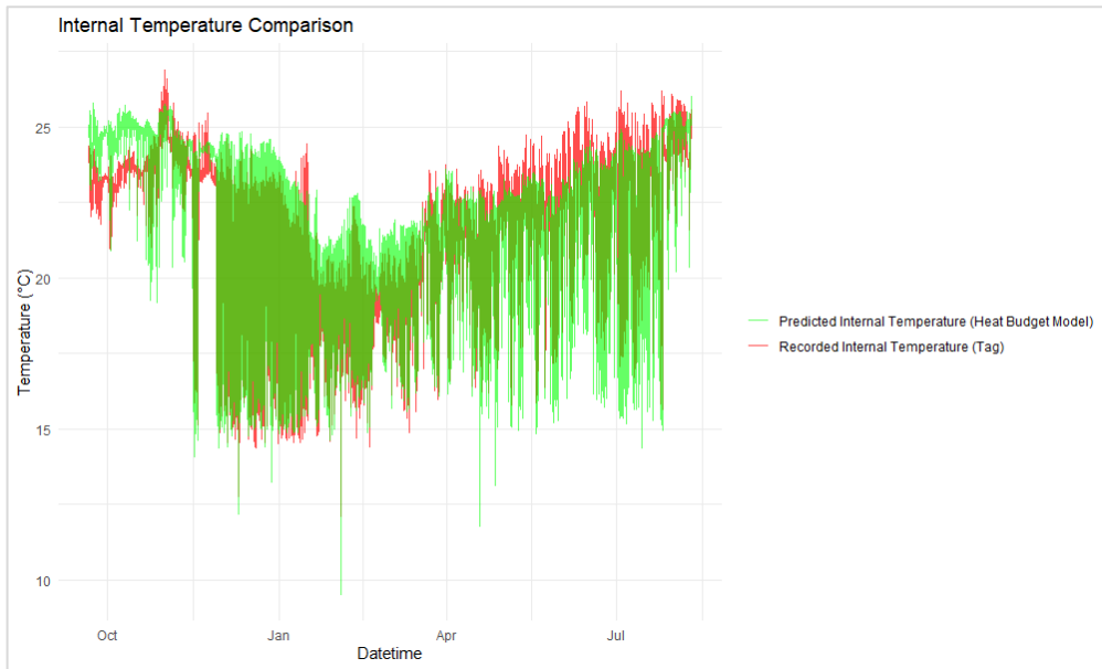
Figure 12. Comparison of recorded internal temperatures (red) and predicted internal temperatures (green) over time.
