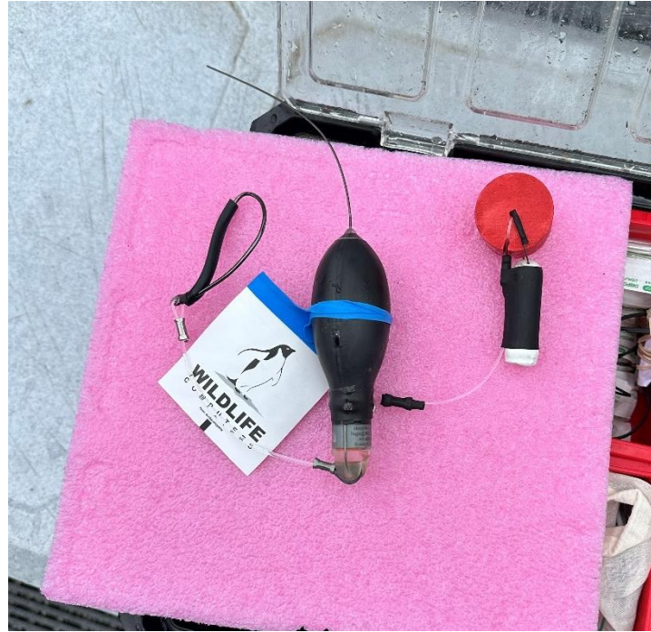
Figure 7 – Insertion hook (on the left); Wildlife Computers pop-up satellite archival tag (in the middle); and conductivity and temperature sensor developed by Star-Oddi (on the right). The picture shows how the CTD was attached to the tag in a novel manner. Photo by the author.
