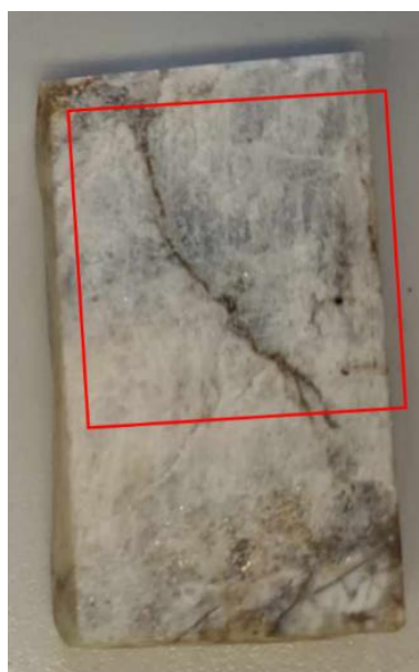
Figure 5.23 – Rock slab containing petalite; the red area indicates the area analysed.
