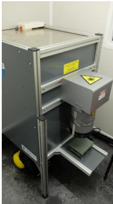
Figure 3.1 – Transportable LIBS system for in-situ operation made for project ¡VAMOS!.
