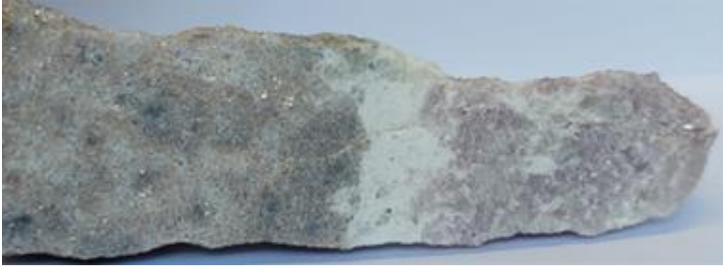
Figure 3.24 – Sample from the Gonçalo pegmatite mine near Guarda, showing three main minerals: zinnwaldite (brown), albite (white) and lepidolite (purple).
