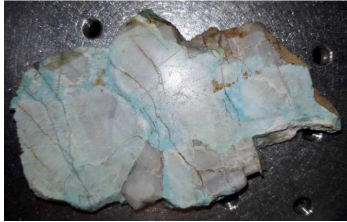
Figure 5.20 – Rock composed of montebrazite, quartz and turquoise, positioned horizontally using a sample holder.
