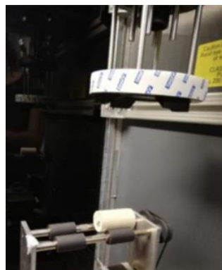
Figure I.1 – Sample holder inserted in the early version of the Nd:YAG system to handle cork stoppers.
