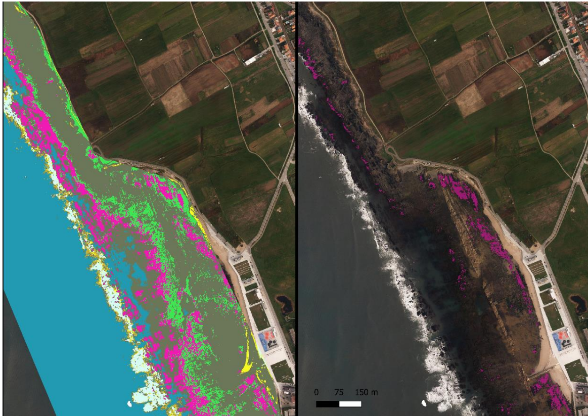
Figure 11: On the left, the map resulting from the initial Land Cover classification, on the right the brown seaweed occurrence map obtaining after the elevation cut-off
