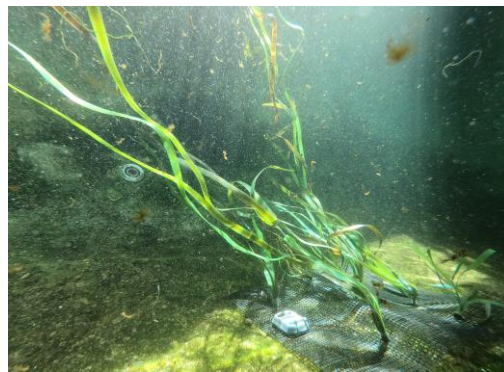
Figure 26. Artificial algae, with approximately one meter in length. The algae were attached to a net and anchored with two weights. This setup prevented the algae from floating to the surface while allowing for easy removal at the end of each observation.
