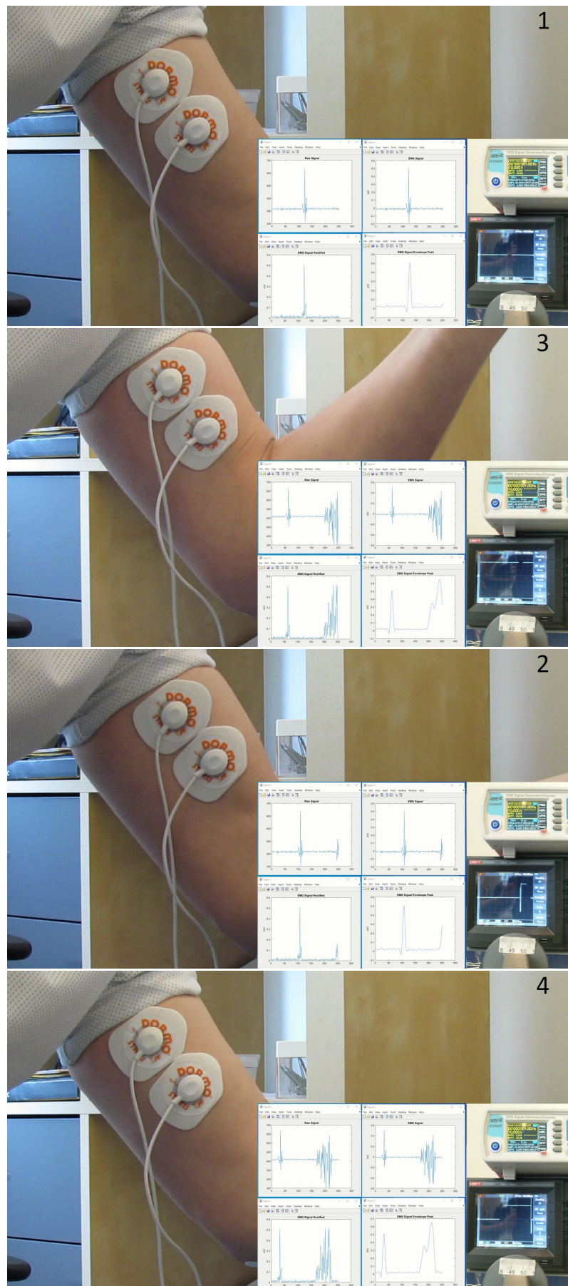
Figure 7.4: Oscilloscope output signal for four sequential instances (different stages) during muscle contraction. 1. 0V without muscle contraction; 2. positive voltage value associated with contraction detection; 3. Stable voltage while contraction is maintained; 4. muscle relaxation induces progressive voltage drop to 0 V.
