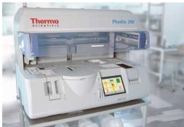
Figura 31. Analisador de ensaios FEIA ( Fluoroenzyme Immunoassay ) ImmunoCAP® 250 da ThermoFisher Scientific (64).
