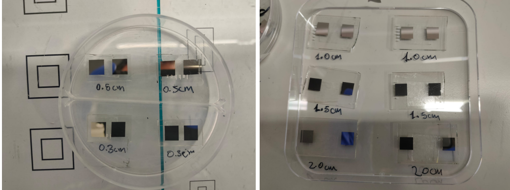
Figure 4.1: Five different configurations of an in-plane TCSC composed of Pt electrodes and PVA/H_3PO_4 electrolyte deposited in a glass substrate.
