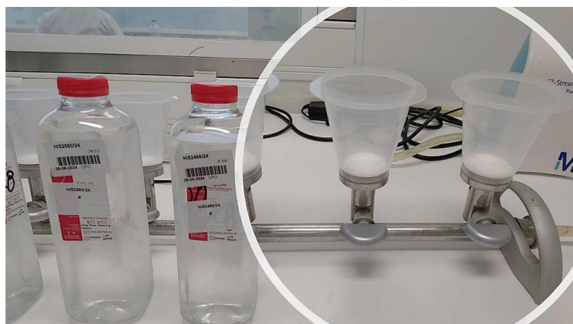
Figure 2 – Final filtration ramp setup with water samples collected in sterile flasks ready to be processed by the membrane filtration method.
