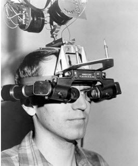
Figure 1.4: First optical head-mounted display built-in 1968 by Ivan Sutherland. (Adapted from [1])
