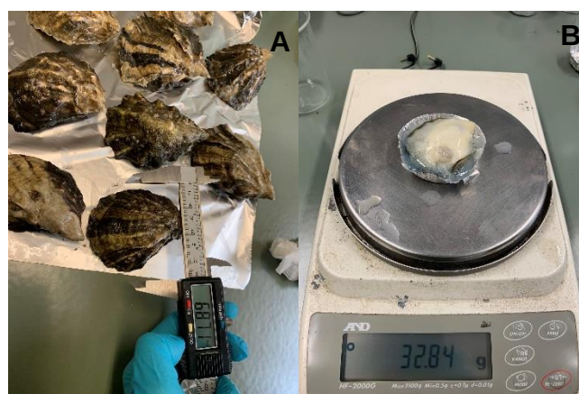
Figure 3. Biometric parameters: (A) digital calliper used to measure the oyster shell length (mm) and (B) digital scale for weighing oyster samples.
