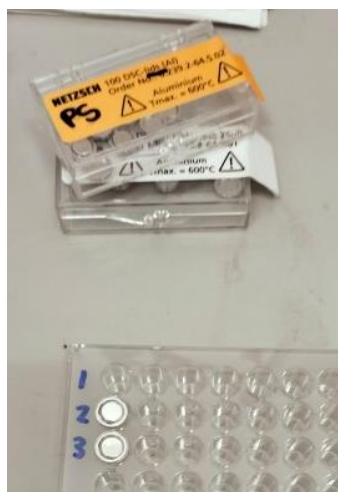
Figure 17. Aluminum crucibles (NETZSCH Premier Technologies, USA) containing CG samples.
