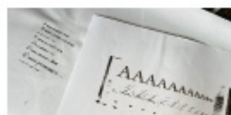
Fig.3. Printing tests with photopolymer matrices and moving characters to prove the quality achieved.
