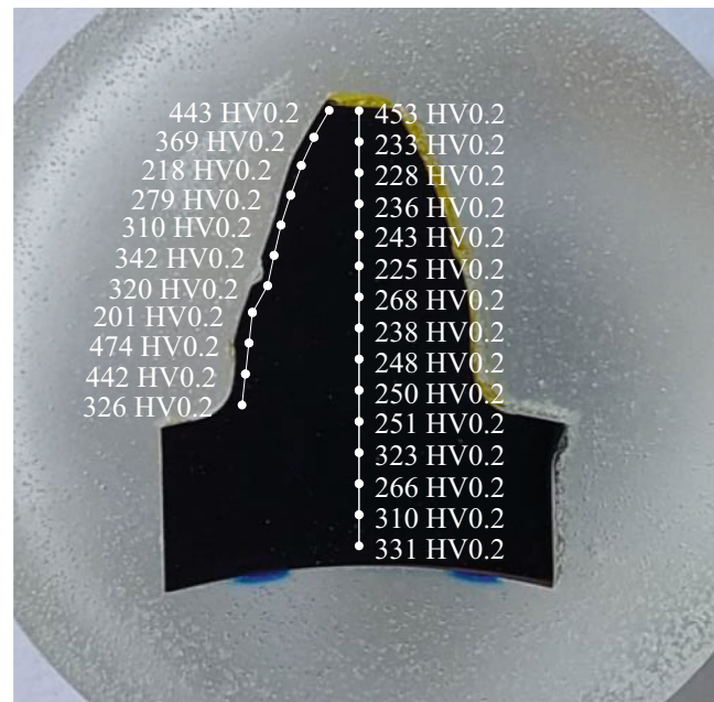
Fig. 14 Tooth 9 cross-section microhardness (HV0.2)
