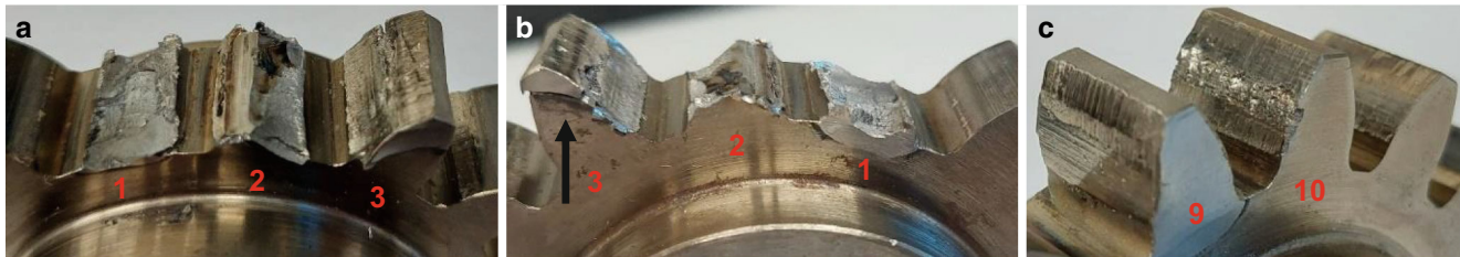
Fig. 19 DLD reconstructed gear after the K14 load stage. a front view for teeth 1, 2 and 3; b back view for teeth 1, 2 and 3; c front view for teeth 9 and 10
