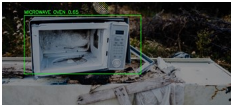
Figure 4.3: Test to validate accuracy and detection of microwave object with trained YOLOv8n model.
