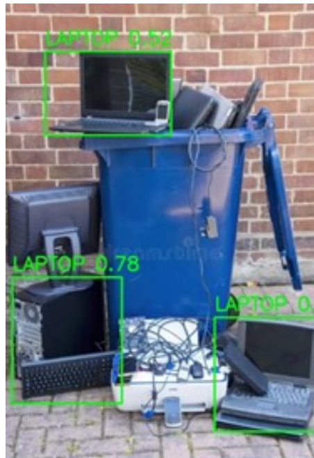
Figure 4.4: Testing to validate accuracy and detection of Laptop object with trained YOLOv8n model.
