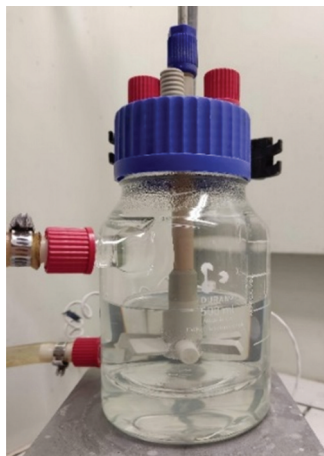
Figure 4. Glass crystallizer used for vanillin crystallization.
