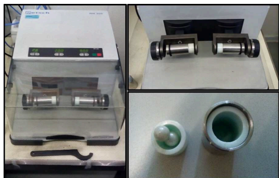
Figure 2. Ball-milling equipment and ceramic pot with ZrO 2 balls.
