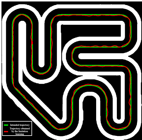
Figure 4.13: Path using Imitation Learning with a state size of 6.
