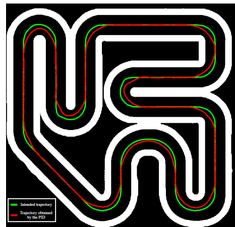
Figure 4.8: Result of the PID controller with a guide line with 80 points of distance between the two endpoints.
