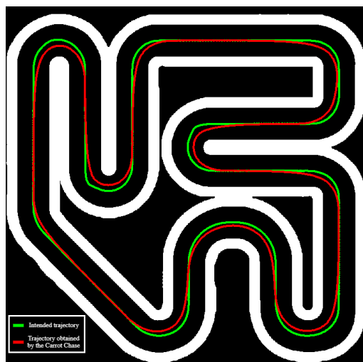
Figure 4.11: Result of the carrot chase algorithm.
