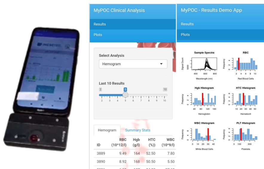
Figure 3.2: POC device connected to a smartphone with the Iot platform represented, showing an example of a blood cell count results and its graphs.
