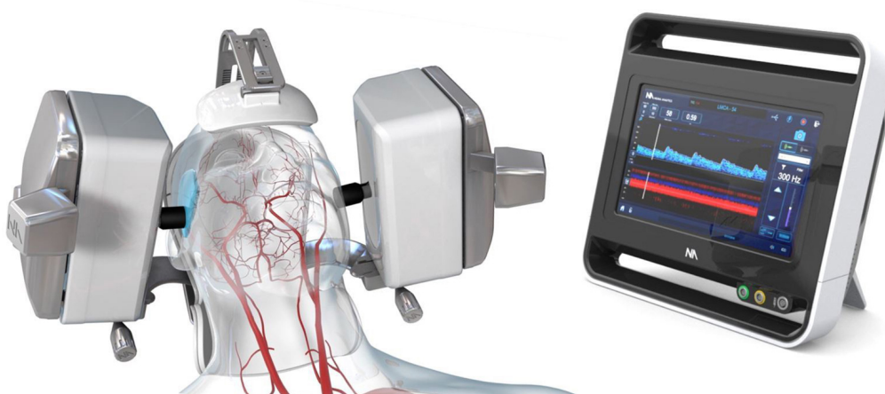
Figure 2.3: The Lucid™ Robotic System (Lucid™ M1 Transcranial Doppler Ultrasound System® and NeuralBot™ System) is a robotically assisted ultrasound system for brain health assessment [39]
