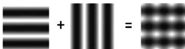
Figure 1.35 - Pattern on a photoresist resulting from the sum of two interference patterns offset by 90°. Adapted from [281]. Copyright 2016 Authors licensed under a Creative Commons Attribution (CC BY 4.0) license.
