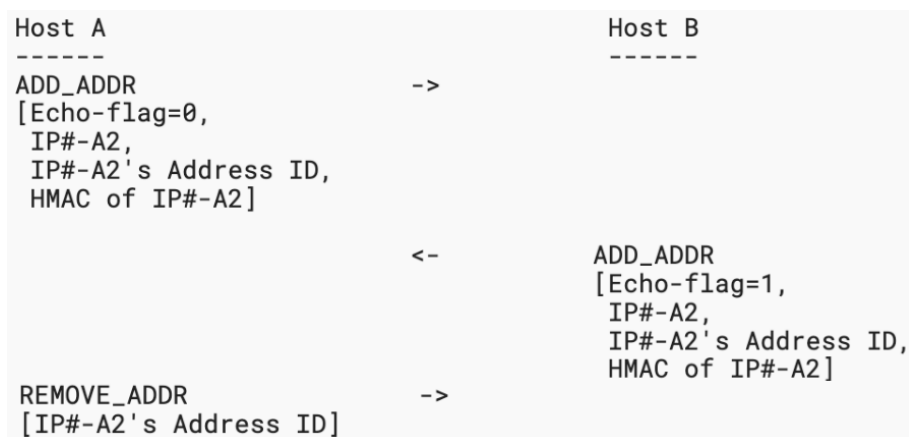
Figure 2.7: Adding a new IP from Host A, interface 2 and removing the same IP. Source: [4].
