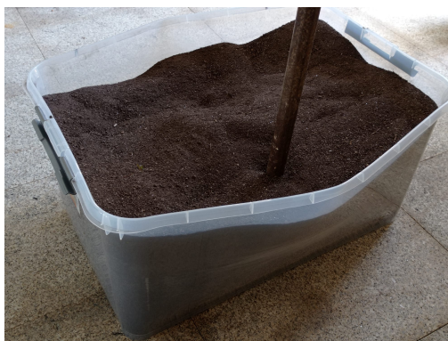
Figure 3.2: Experimental setup using plastic box filled with soil. Objects were buried vertically and GPR scans were taken on the biggest side wall.
