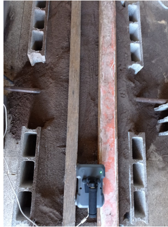
Figure 3.4: Experimental setup used for the verification of the system. Objects were buried horizontally and GPR scans were taken along the soil's surface considering a height offset
