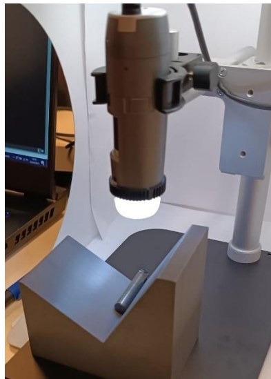
Figure 4.4: Dino-lite capture of a solid milling tool after a milling operation.
