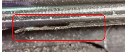
Figure 5.20: Burr found at 790 mm of cut length when machining in a linear strategy.
