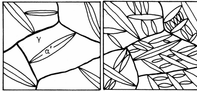
Figure 2.7: Schematic of the growth of \alpha' -martensite plates [28].
