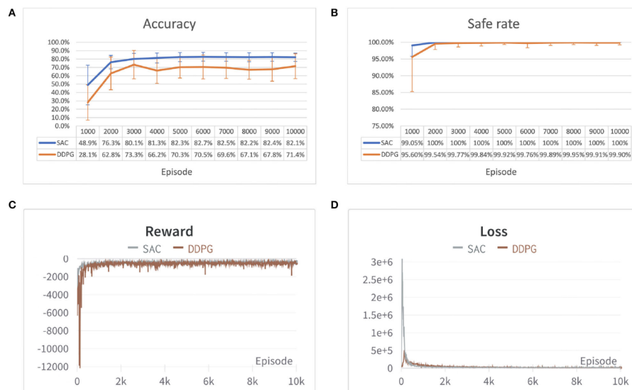
Figure 2.13: Accuracy and Safe-Rate comparison between SAC and DDPG across different episodes in a Path Planning task optimizing the movement of a robotic arm, taken from Chen et al. (2022) .
