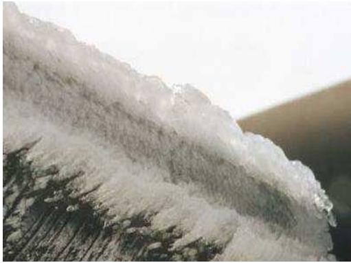
(a) Mixed ice formation on an aircraft wing [32].
