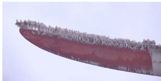
Figure 2.3: Rime ice formation on a wind turbine blade [28].
