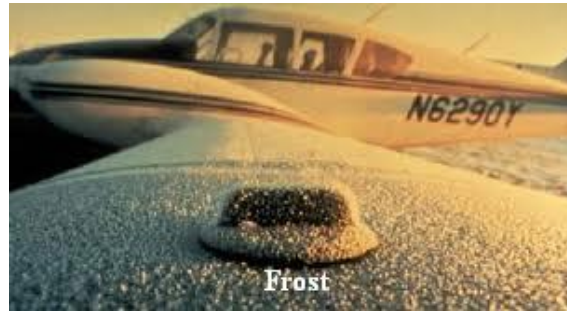
Figure 2.5: Frost formation on an aircraft wing [31].
