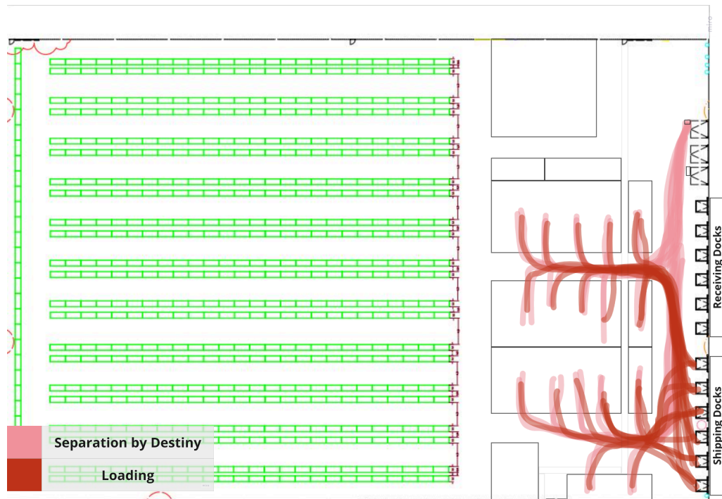
Figure 16 - Spaghetti Diagram of the Expedition process of the EDC Factory Operation
