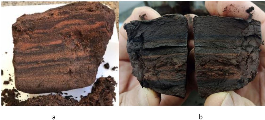
Figure 18 – Example of layered block sample of Brumadinho tailing Dam (Arroyo & Gens, 2021)
