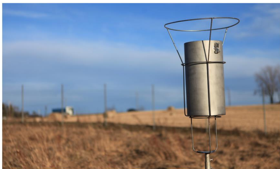
Figura 1-Amostrador do tipo passivo, innovation NILU AS Fonte: https://innovation.nilu.no/wp-content/uploads/sites/14/2020/04/innovation_nilu_Atmospheric_Microplastic_Collector_2020.pdf
