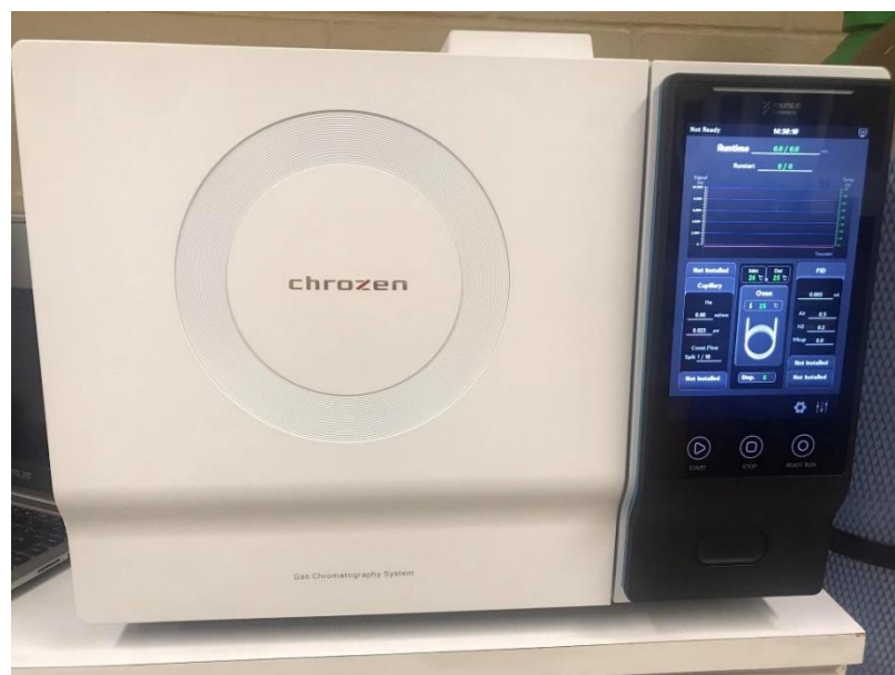
Figura 6-Sistema GC-FID, Chrozen GC
