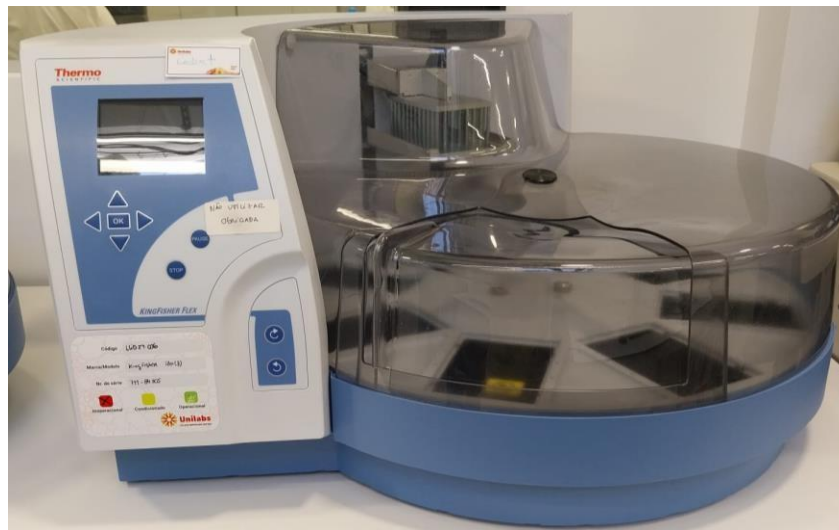
Figure 3. Image representing the KingFisher™ Flex Magnetic Particle Processor with 96 Deep-Well Head.
