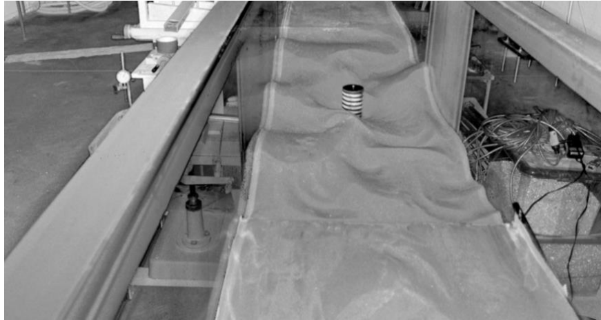
Figure 45. Live-bed regime in test with critical velocity equal to 0.24m/s
