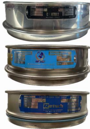
Figure 29. Sieves of 0.115, 1 and 2.36 mm used
