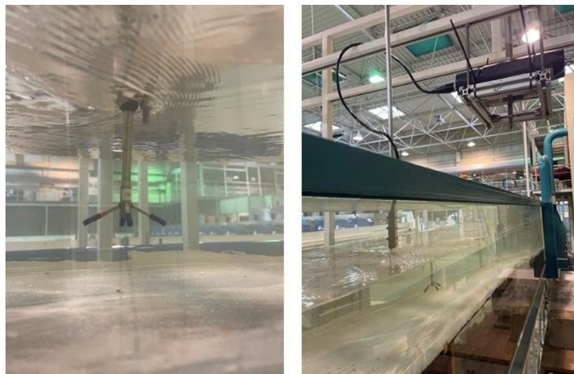
Figure 33. ADV and support structure
