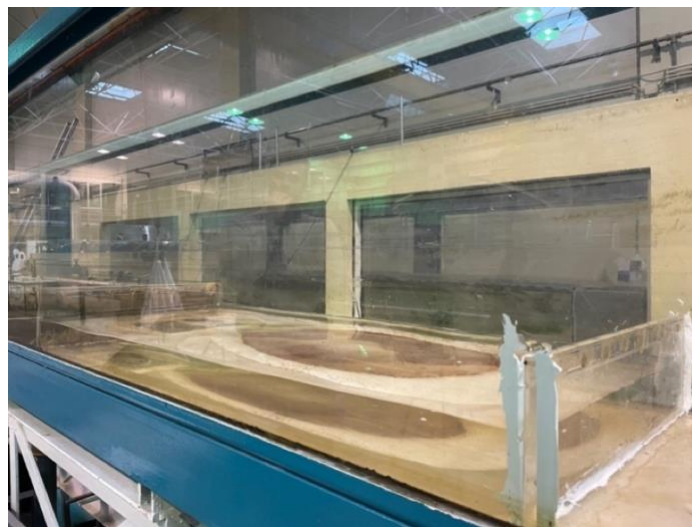
Figure 25. Sediment retention chamber
