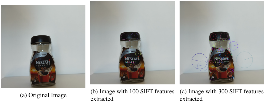
Figure 4.6: Extraction of SIFT Features
