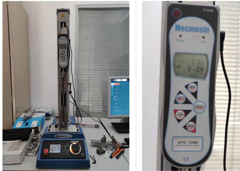
Figure 4.8: Equipment used to perform the uniaxial tensile tests: MultiTest 2.5-dV (left) and AFG of 100 N (right).
