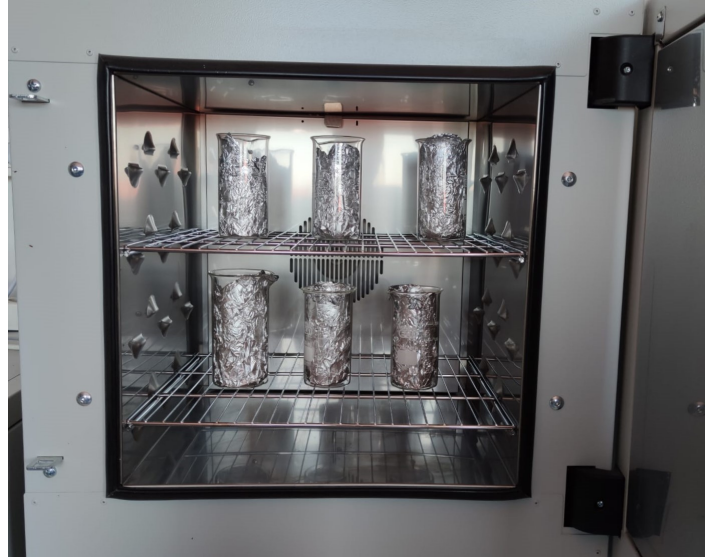
Figure 4.2: Samples inside the Drying Oven VWR® VENTI-LINE® for melt-blending the material.
