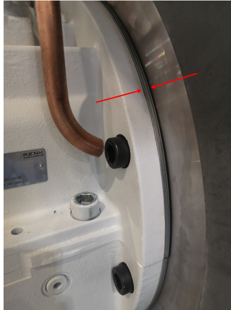
Figure 4.2: Shims on non-flameproof motors for axial alignment
